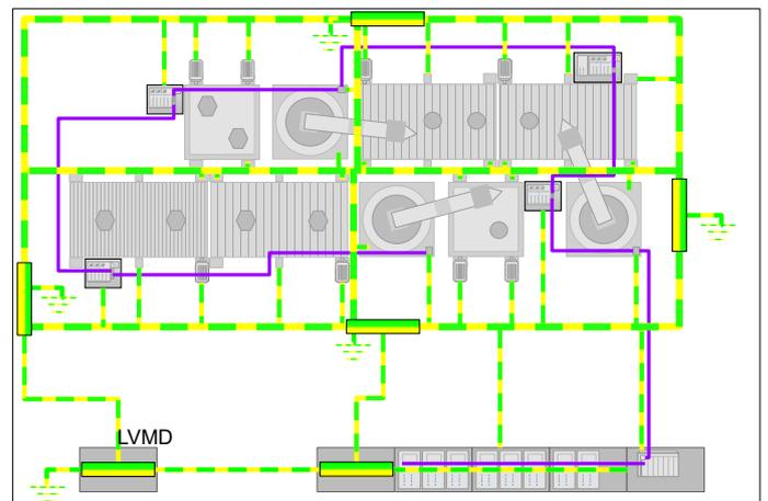
FIGURE 9: Meshed equipotential bonding system (MESH-BN)
