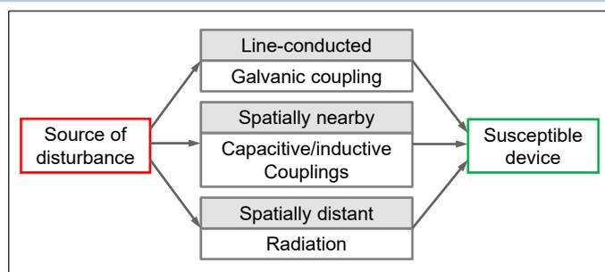
FIGURE 1: Coupling types between source of disturbance and a susceptible device
