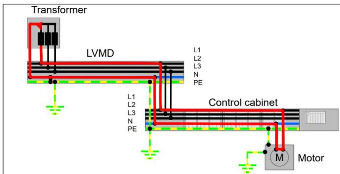
FIGURE 7: TN-S system with load and current flow
