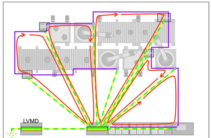
FIGURE 8: Meshes in an equipotential bonding system with star topology through cable shielding
