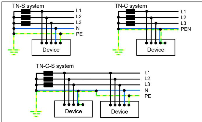
FIGURE 5: Network structures TN-S, TN-C and TN-C-S
