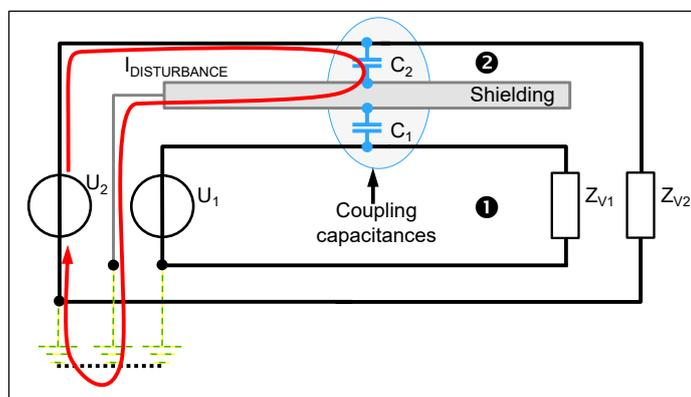
FIGURE 3: Shielding as a measure against capacitive coupling
