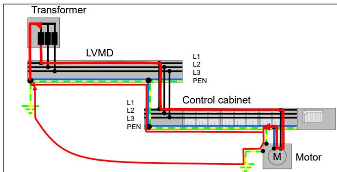
FIGURE 6: TN-C system with load and current flow
