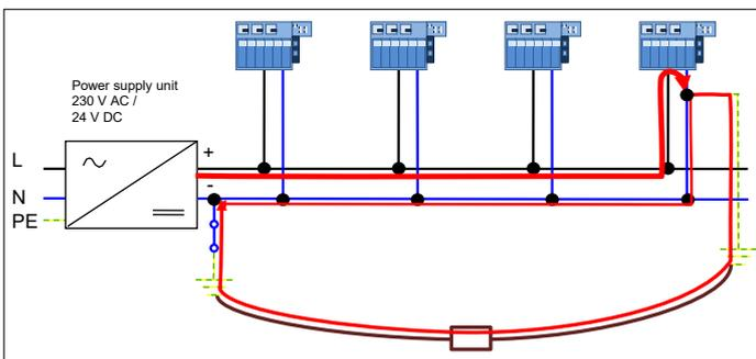
**FIGURE 12:** Multiple grounding of a 24 V supply circuit
