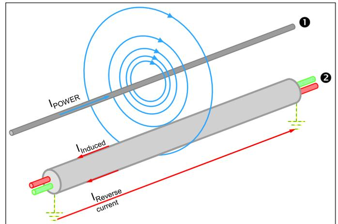
FIGURE 4: Induction in the cable shielding
