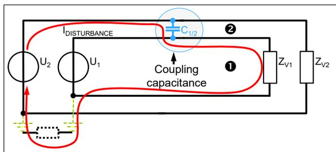
FIGURE 2: Capacitive coupling between two circuits
