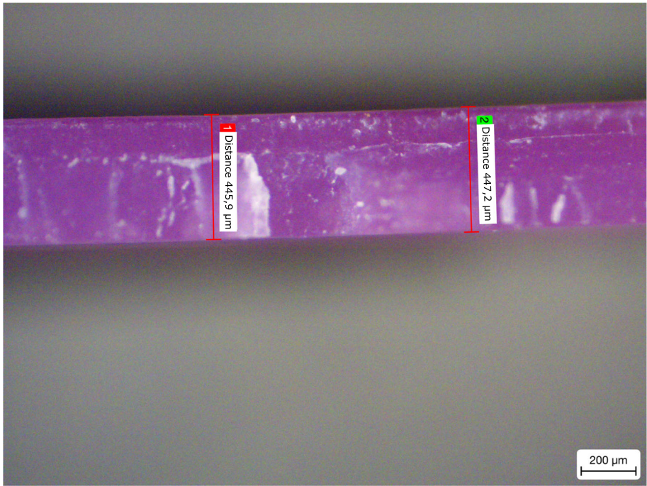
Fig. 8 Microscopic image of [\text{Fe}(\text{atrz})_3]\text{Cl}_{1.5}(\text{BF}_4)_{0.5} in Polystyrene
