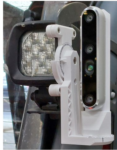
Figure 4. A stereo camera mounted to a forklift.
